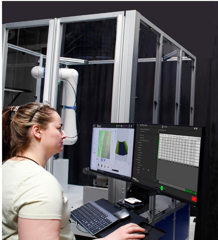
Figure 1. An inspector reviewing pass-fail results from an automated measurement system.
