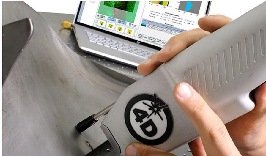
Figure 2. A 4D InSpec optical gage measuring feature depth on a complex geometry.
