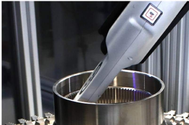
Figure 4. Measure in challenging locations: between fir tree roots and inside of a bore.
